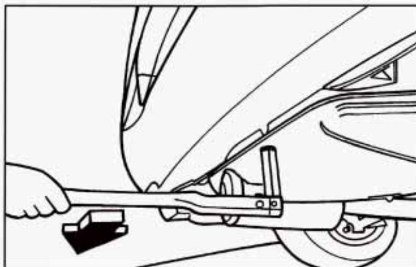
The spare tire is on a tire carrier tray under the rear end of your vehicle. See "Compact Spare Tire" later in this section for more information about the compact spare. To lower the tray, position yourself behind the vehicle facing the front and use the socket end of the wheel wrench to turn the latch bolt clockwise. Lower the tray about 1 inch (25.4 mm). Don't loosen the latch bolt too much, or the tray could fall.
