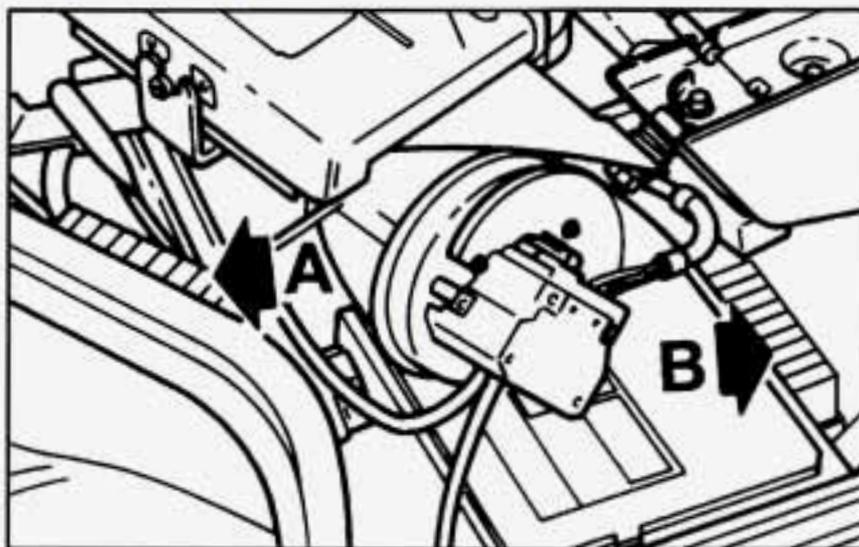
There are two maxi-fuse blocks in the engine compartment. One is part of the forward lamp wiring harness (A), and the other is part of the ECM-engine wiring harness (B).
