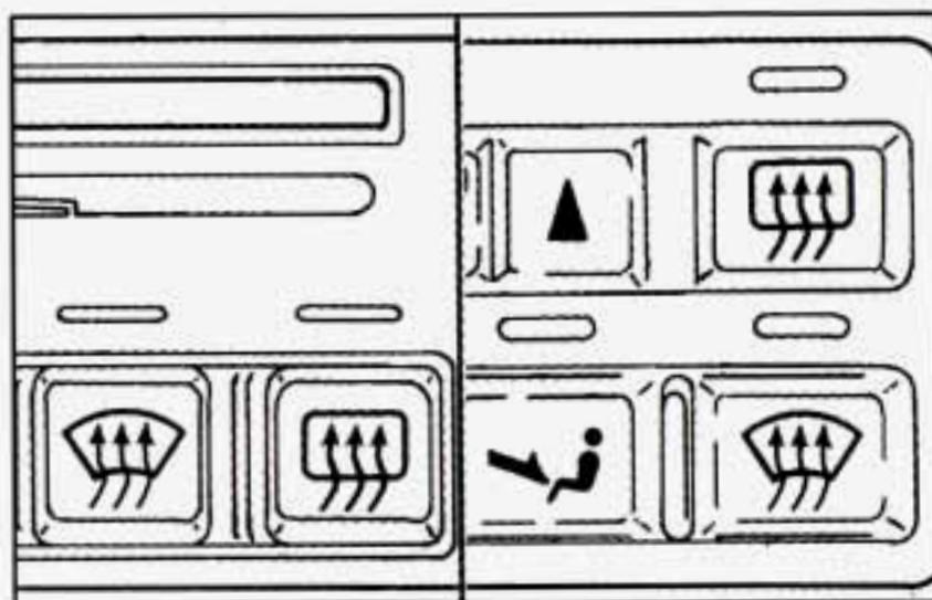
The rear window defogger uses a warming grid to remove fog from the rear window. The power mirrors are also warmed when the rear window defogger is on.
