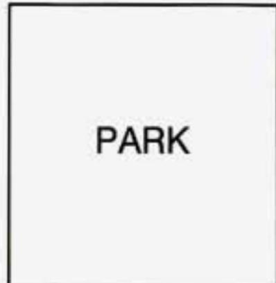
When the ignition is on, this light will come on when you set your parking brake. The light will stay on if your parking brake doesn't release fully.
