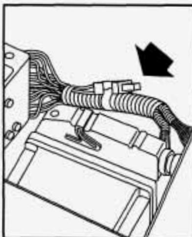
Vehicles equipped with the optional Real Time Damping ride control system are fuse protected with a fuse located in the ABS compartment behind the driver's seat.
