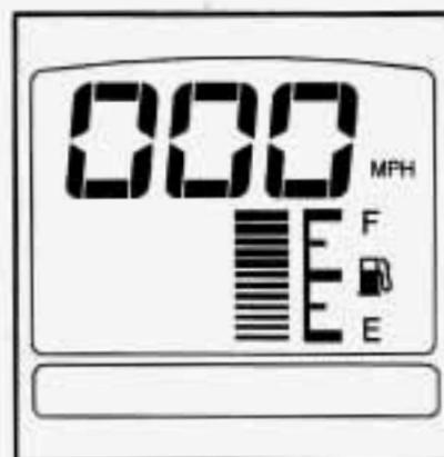
Your fuel gauge shows about how much fuel is in your tank. The bars light up when the ignition is on or, if the ignition is off, when you turn on your parking lamps.
