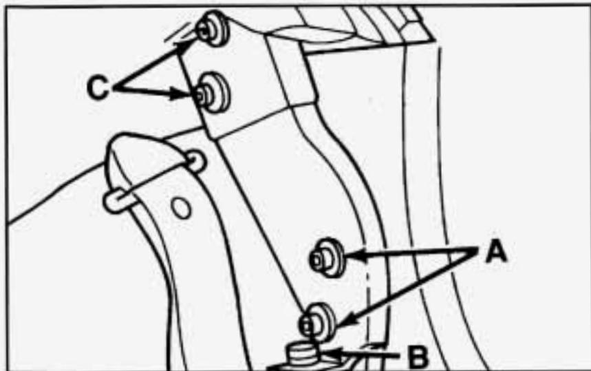
5. Using the wrench, remove the two lower bolts (A) from the lock pillar bracket on each side.
