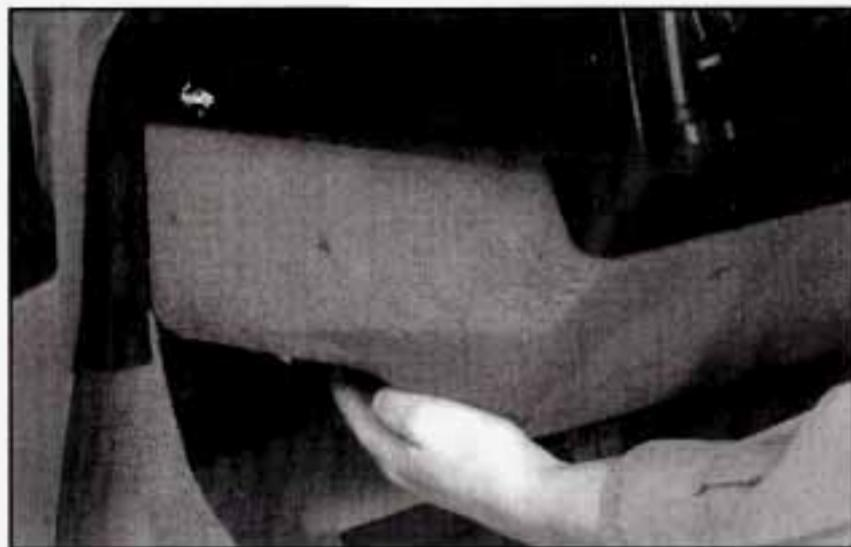
To open the hood, first pull the handle inside the vehicle.
