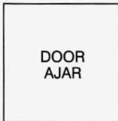
This light comes on when you open one of the doors with the ignition on. It stays on until you fully close the door. Have your vehicle serviced if the light comes on and stays on, even when the doors are fully closed.
