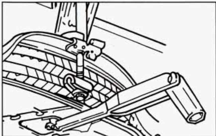
Put the hooked end of the wheel wrench into the slot in the tray. Insert the wheel wrench a little from the side so it isn't over the latch bolt. Pull up on the wheel wrench to lift the tray.
