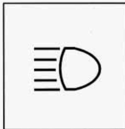
To change the headlamps from low beam to high or high to low, pull the turn signal lever all the way toward you. Then release it. When the high beams are on, this light on the instrument panel also will be on.
