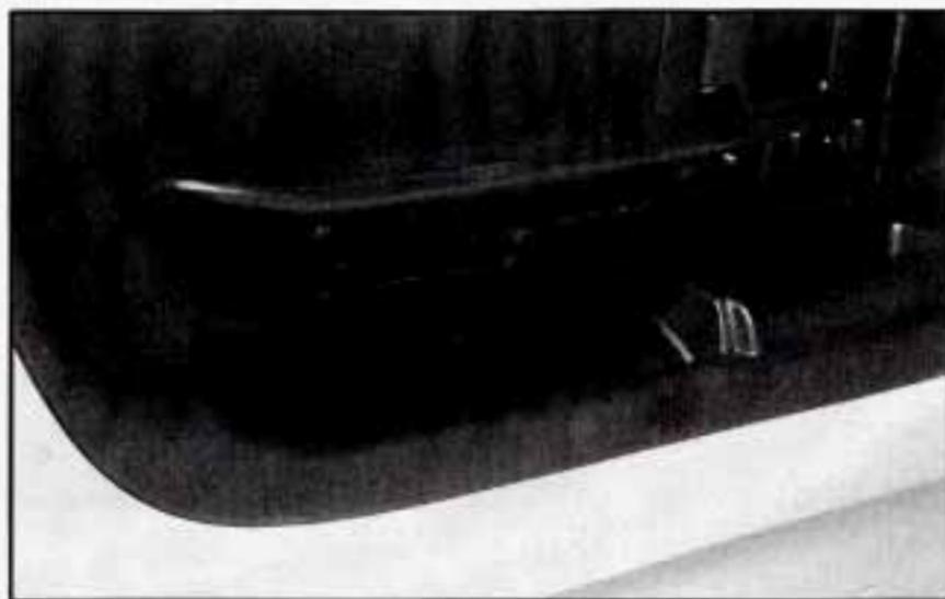
Each door has a storage compartment below the armrest which can be accessed by lifting up on the armrest.
