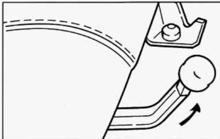
Move the lever under the front of the seat to unlock it. Slide the seat to where you want it. Then release the lever and try to move the seat with your body, to make sure the seat is locked into place.
