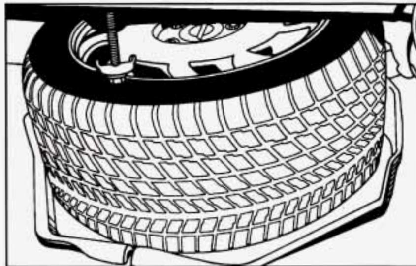
Put the tire on the tray. For the flat road tire, lift the latch bolt, pull it toward the rear of the vehicle, and the bolt will drop down to the lower position. For the spare tire, push up the latch bolt and push it toward the front of the vehicle to raise it to the upper position.
