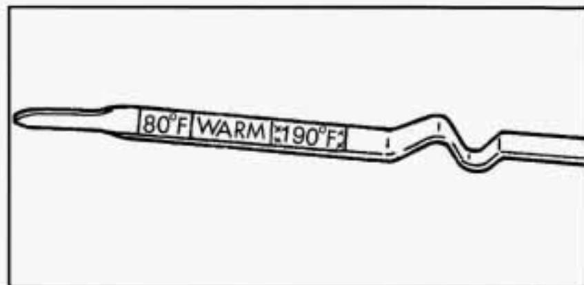
3. Check both sides of the dipstick, and read the lower level. The fluid level should be in the area marked "80°F" for a cold check and will move into the "WARM" area as the temperature increases. When the fluid is at normal operating temperature (180°F to 200°F, 82°C to 93°C), the level must be in the crosshatched area marked "190°F." See "Automatic Transmission Fluid Temperature Reading" in the Index.
