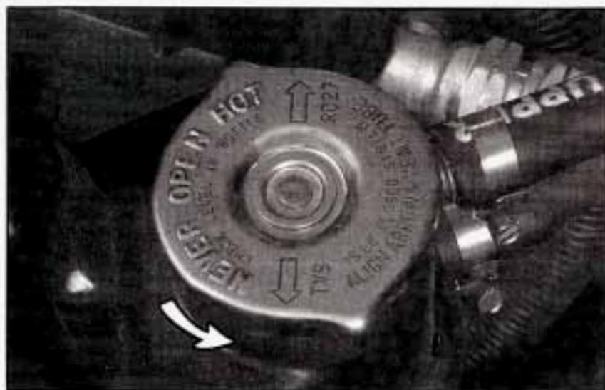
1. You can remove the coolant high fill reservoir pressure cap when the cooling system, including the coolant high fill reservoir pressure cap and upper radiator hose, is no longer hot. Turn the pressure cap slowly counterclockwise until it first stops. (Don't press down while turning the pressure cap.)
