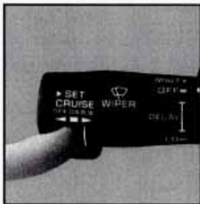
Once you're going about 25 mph (40 km/h) or more, you can move the cruise control switch to R/A (Resume/Accelerate) for about half a second.
