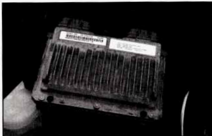
You must loosen and remove the two screws before the PCM unit will lift out.
