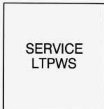
The SERVICE LTPWS light comes on whenever a LTPWS part is not working properly. It may also come on when you're going less than 25 mph (40 km/h) or in stop-and-go traffic.
