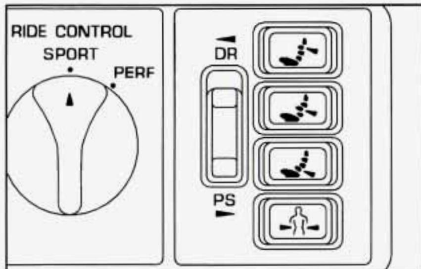
These switches let you change the shape of your seat. There are three lumbar supports for the upper, middle and lower back. There's also a side bolster that adjusts the sides of the seat around you to give you more lateral support.
