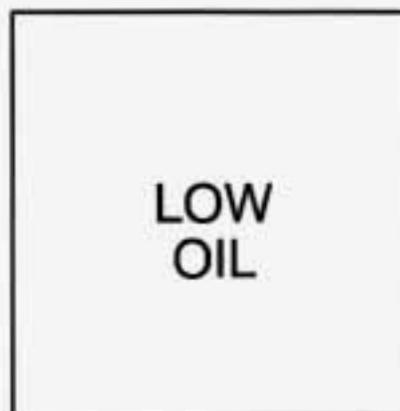
This light should come on while you are starting your engine. If the light doesn't come on, have it repaired. If the light comes on while starting your engine and stays on, your engine oil level may be too low. You may need to add oil. See "Engine Oil" in the Index.
