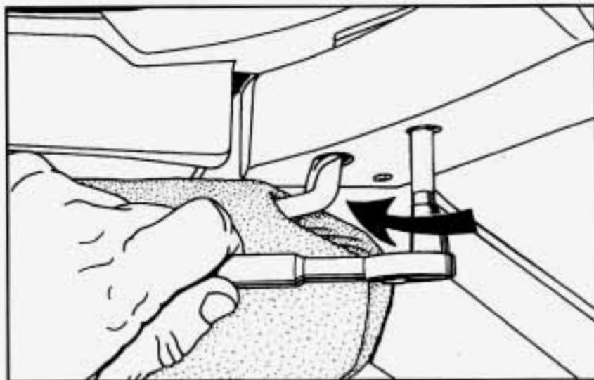
2. Loosen the front bolts with the wrench.
