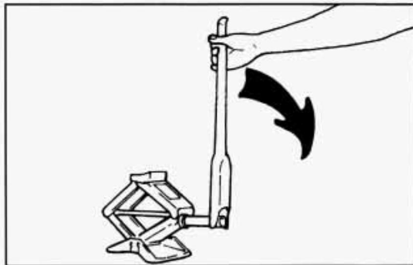
4. Attach the wheel wrench to the jack. Hold the wheel wrench handle so it forms a right angle with the jack, then turn it clockwise.
