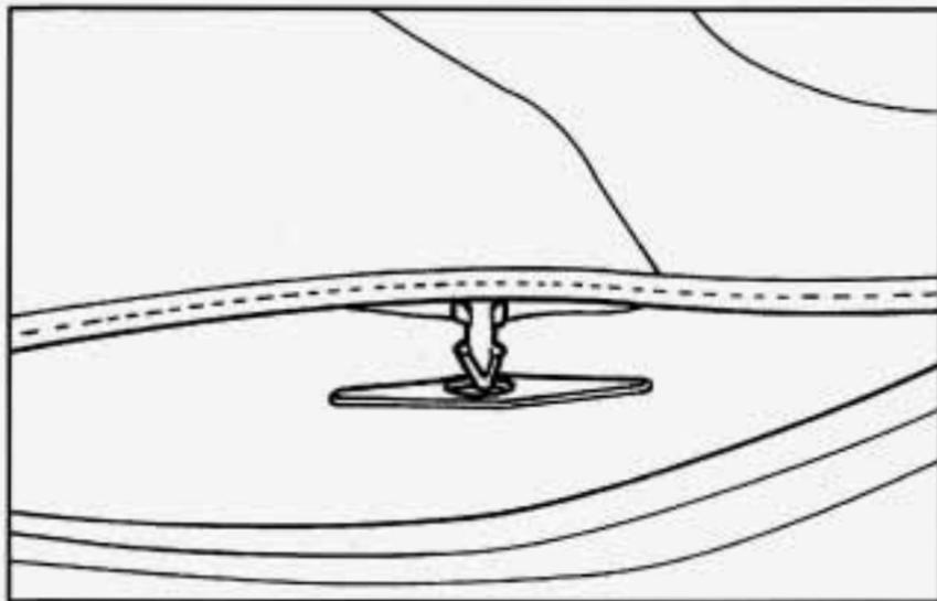
6. Lower the rear of the top so the latch pins align with the holes in the lid. To secure the rear of the top, push down firmly on both corners.
