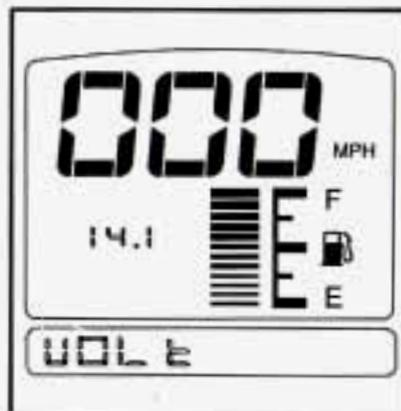
For numeric gauge measurements, press the GAUGES button on the trip monitor until VOLT appears. The number that appears next to the fuel gauge is the battery voltage.
