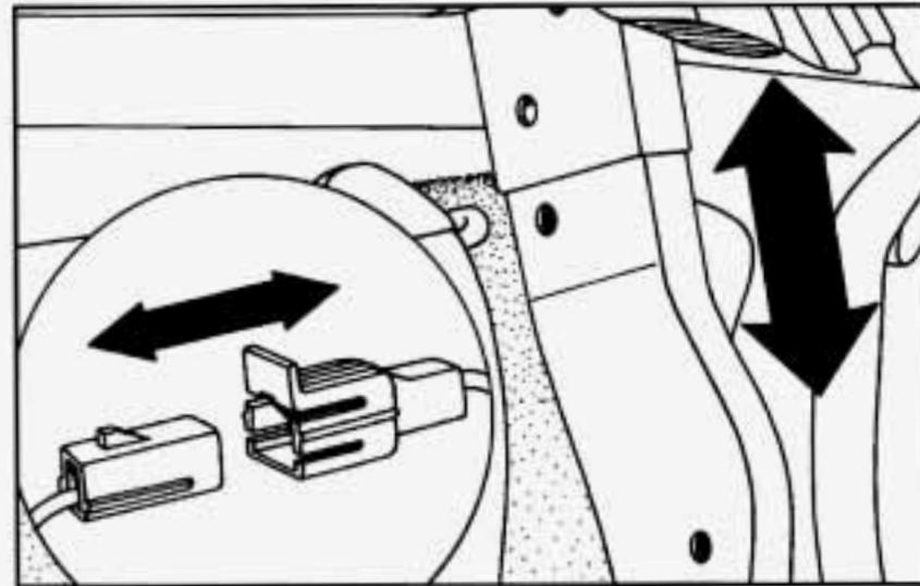
8. Slide both lock pillar brackets down and forward from the receiver brackets. You may need to lift the hardtop slightly to remove the brackets.
