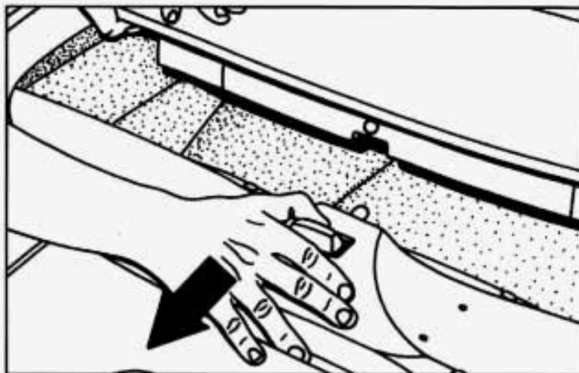
2. Store the roof panel with its top up and its rear pointing forward. Slide the rear corners of the roof panel into the brackets and push forward.
