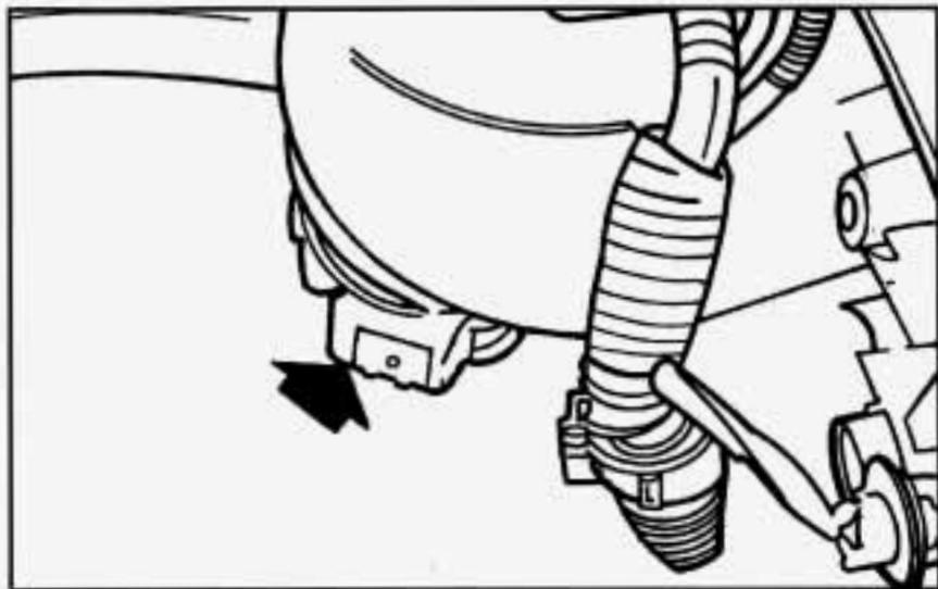
You can reach the front cornering lamp from inside the engine compartment.
