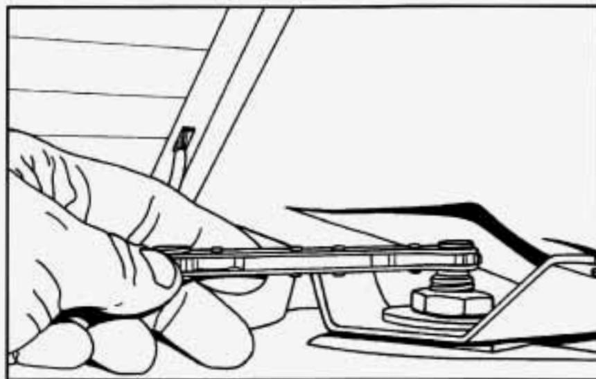
4. Loosen the rear corner bracket bolts with the ratchet.
