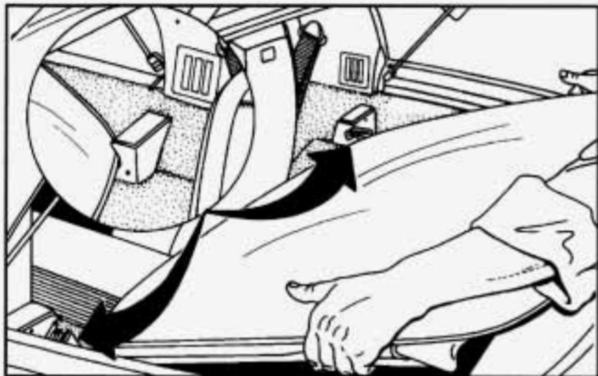
1. Open the rear hatch and look for the two brackets in the rear area. The brackets are below the courtesy lamps.
