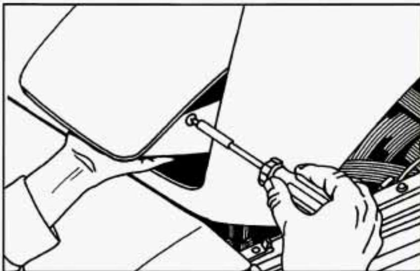
4. Remove the two screws from both sides of the cover. Before you remove the last screw, put your hand under the cover to hold it.
