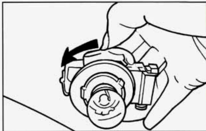
2. Push the bulb in, turn it counterclockwise, then pull it out.
