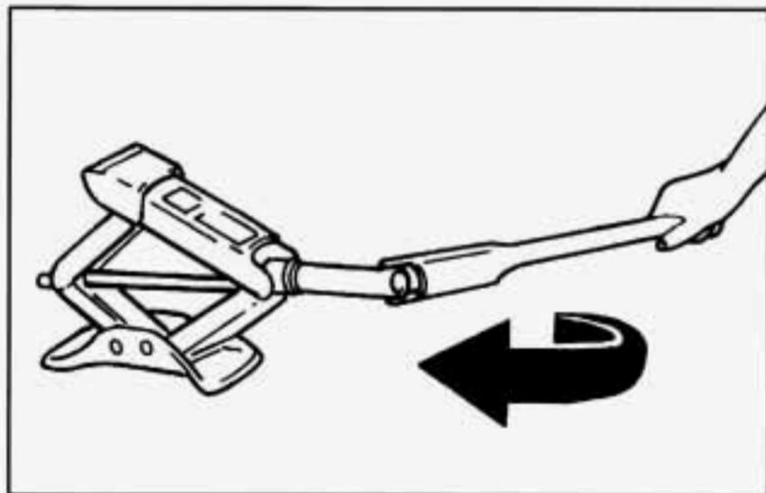
5. When you've turned the wrench almost as far as it will go, swing it around to the other side. Keep turning to raise the jack lift head a 3 inches (76.2 mm).
