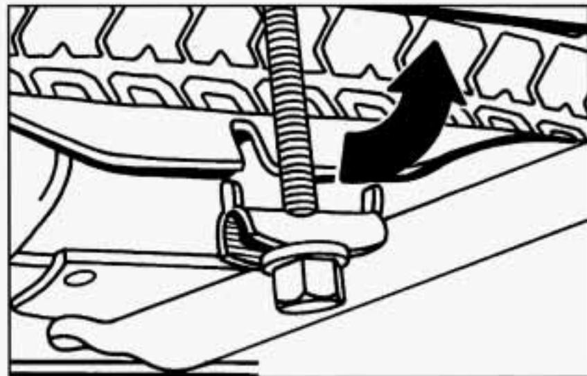
While holding the tray up with the wheel wrench, pull the latch bolt rearward to release it from the tray. If it won't come free, loosen it a little more.
