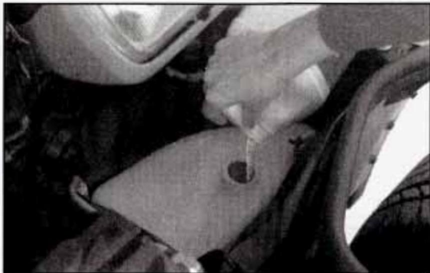
10. Then fill the coolant recovery tank to the proper level. For a complete drain, flush and refill, see your Chevrolet dealer or a Chevrolet Corvette Service Manual. To purchase a service manual, see "Service and Owner Publications" in the Index.
