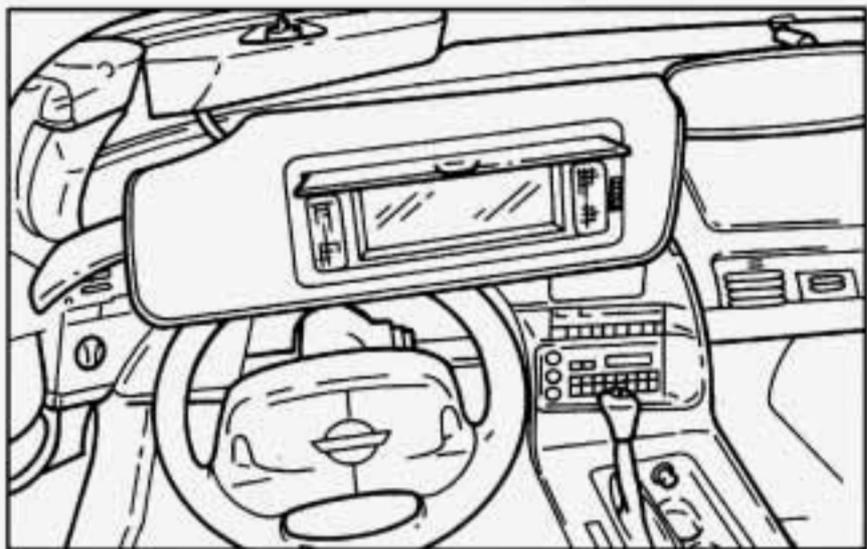
Pull down the sun visor and lift the cover to expose the vanity mirror. When the ignition is on, slide the switch next to the mirror up to turn the lamps on. Be sure to turn the lamps off before closing the cover.
