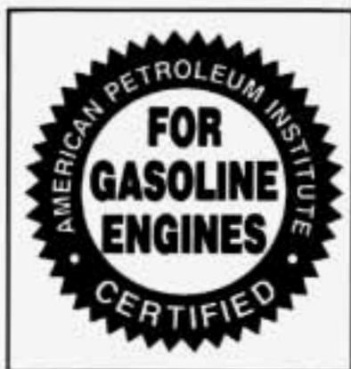
Oils meeting these requirements should also have the “Starburst” symbol on the container. This symbol indicates that the oil has been certified by the American Petroleum Institute (API). Do not use any oil which does not carry this Starburst symbol.
