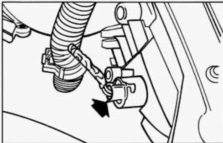
You can reach the front sidemarker lamp from inside the engine compartment.
