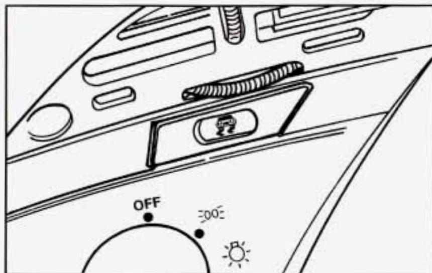
To turn the system off, press the button located above the headlamp switch. The ASR OFF light will come on and stay on. If the ASR system is limiting wheel spin when you press the button, the system will turn off right away.
