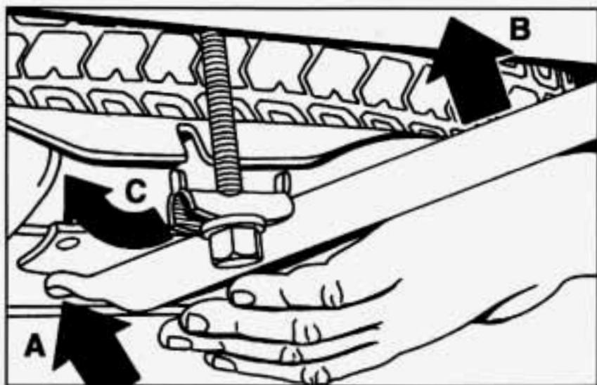
Put the hooked end of the wheel wrench into the slot in the tray (A). Lift the tray using the wheel wrench (B) and insert the latch bolt into the notch in the tray (C). To raise the tray, use the socket end of the wheel wrench to turn the latch bolt counterclockwise. Turn the latch bolt until it is snug.
