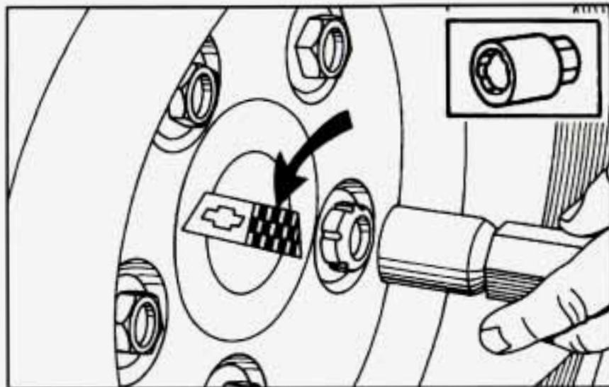
2. Each wheel will have one locknut. A special wheel lock key (removal tool) and instructions are provided. Attach the wheel lock key to the wheel wrench. Remove the locking wheel nut by turning counterclockwise.
