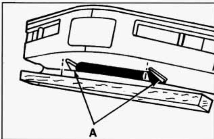
Position a 4" × 4" wood beam across sling chains contacting under fascia just ahead of the curb protect brackets (A).
