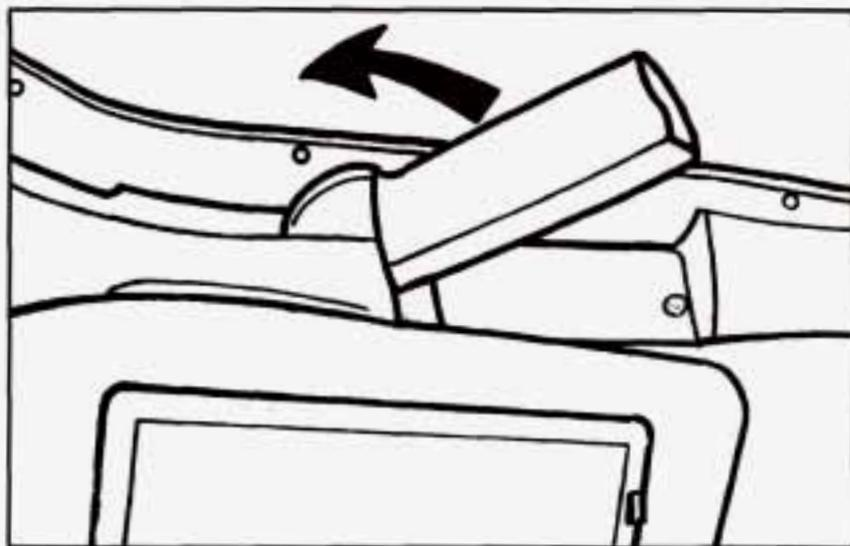
2. Unlock the front of the convertible top by turning the latch handles outward. Then lift the top off the windshield slightly.
