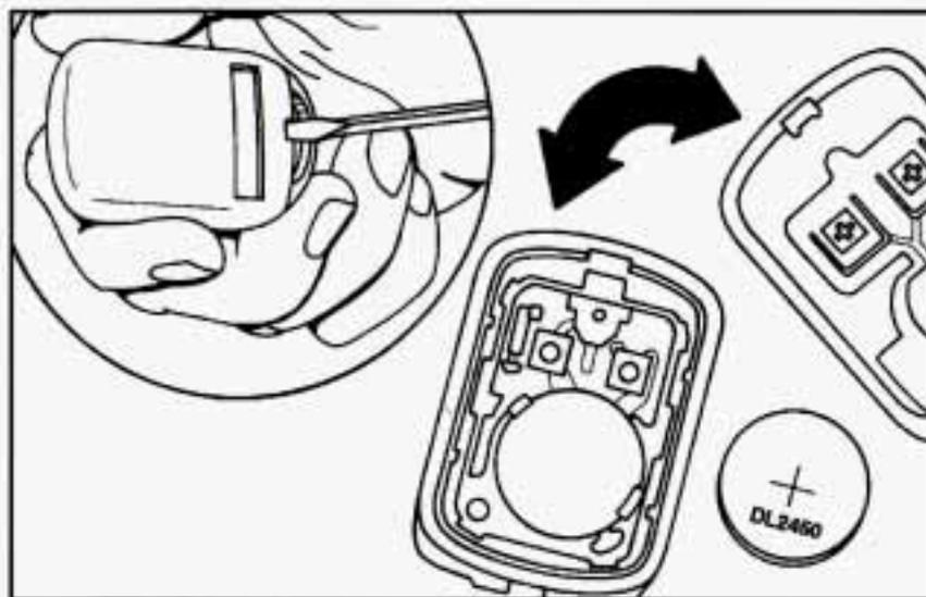
1. Insert a screwdriver into the slot on the back of the transmitter and gently pry apart the front and back.
