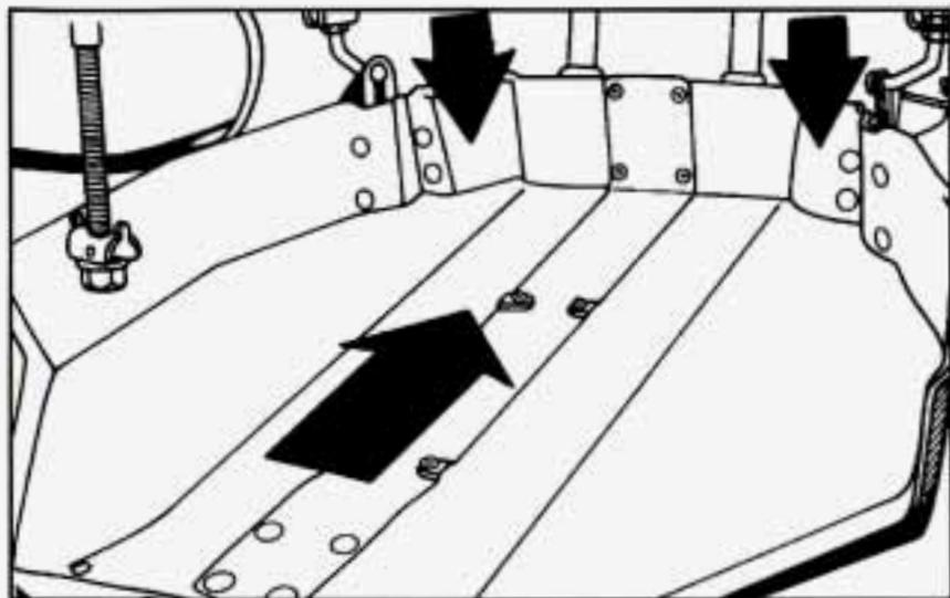
If your vehicle is equipped with a spare tire, the road tire is larger than the spare, so you must adjust the tray to its lower position. Lift and push the tire carrier tray toward the front of the vehicle. The tray will drop to its lower position.
