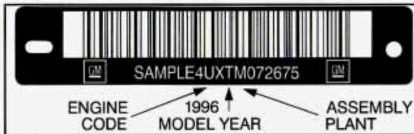
This is the legal identifier for your Corvette. It appears on a plate in the front corner of the instrument panel, on the driver's side. You can see it if you look through the windshield from outside your vehicle. The VIN also appears on the Vehicle Certification and Service Parts labels and the certificates of title and registration.
