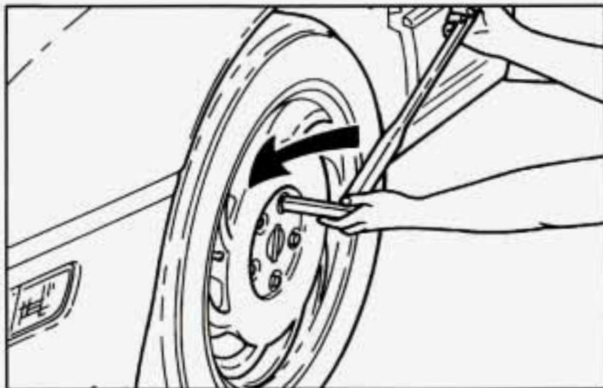
1. Remove the plastic wheel nut caps using the socket end of the wheel wrench by turning the wrench in the direction shown. Store the caps somewhere until you have the flat tire repaired or replaced.
