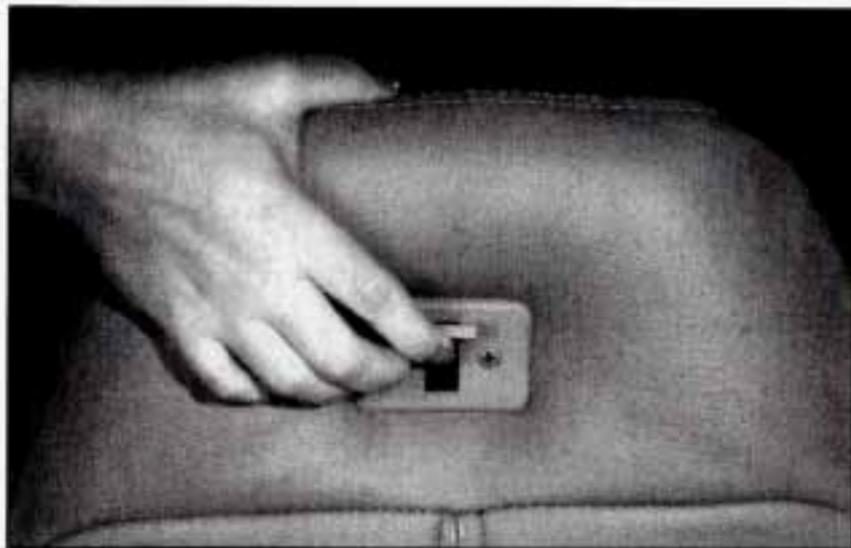
Both seatbacks fold forward to give you access to the rear area. To fold a seatback forward, lift this latch and push the seatback forward. When you return the seatback to its original position, make sure the seatback is locked.
