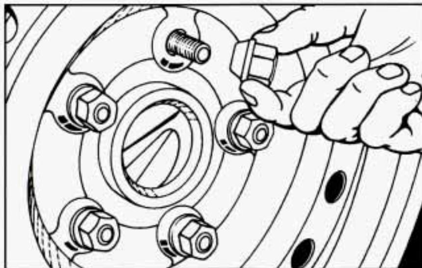
9. Replace the wheel nuts with the rounded end of the nuts toward the wheel. Tighten each nut by hand until the wheel is held against the hub.
