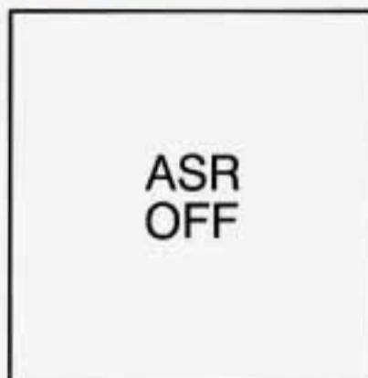
This light will come on for a few seconds when you turn the ignition on. It also comes on and stays on when the ASR button is pressed to turn the system off.
