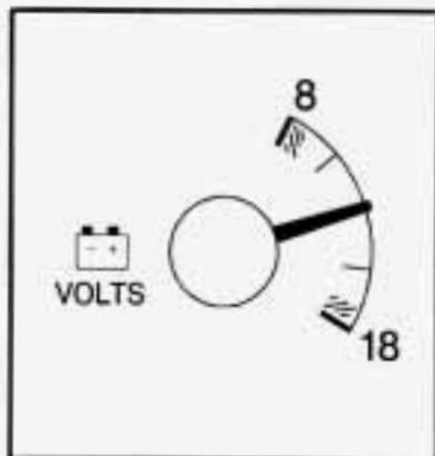
When the engine is not running, the voltmeter shows the voltage output of your battery. When the engine is running, it shows the voltage output of the charging system.
