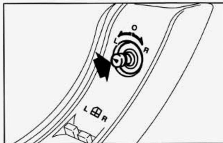
The electric mirror control is on the driver's door. To adjust either mirror, turn the switch to LEFT (L) or RIGHT (R). Then use the control to adjust the mirror. When you are done adjusting the mirrors, move the control back to the center to avoid accidental adjustment.
