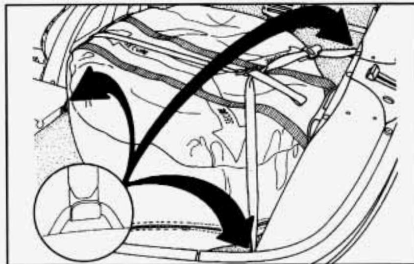
A Grand Sport Coupe rear tire will not fit in the tray, so you must put it on the floor of the rear area. Put the flat tire in the storage bag provided with the spare. Place the tire on the rear area floor.
