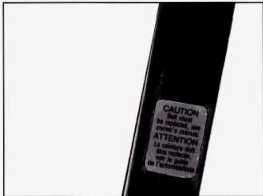
If you ever see a label on the passenger's safety belt that says to replace the belt, be sure to do so. Then the new belt will be there to help protect you in a collision. You would see this label on the belt near the latch plate.
