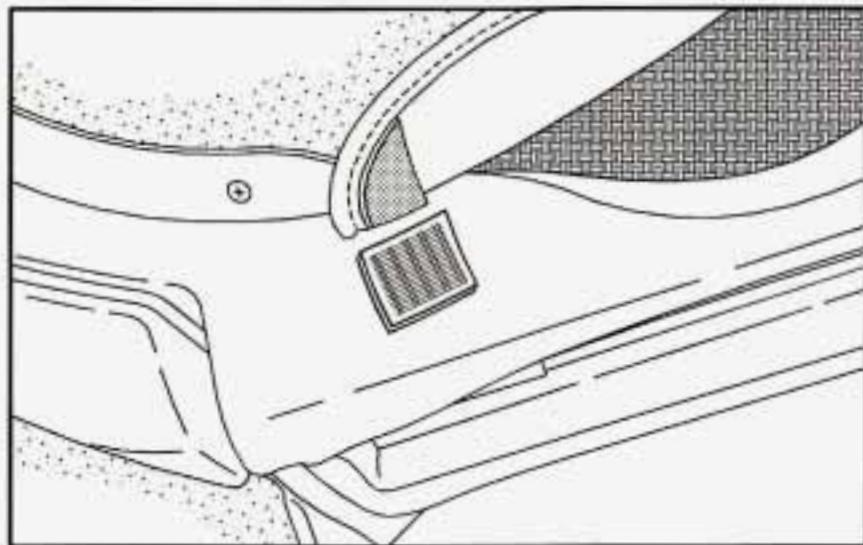
7. Fasten the strips for the headliner at the rear of each window opening.
