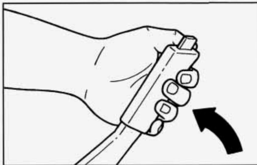
To set the parking brake, hold the brake pedal down. Pull the parking brake lever up, then move it back down. This sets your parking brake, even though the lever is down. If the ignition is on, the parking brake indicator light will come on.
