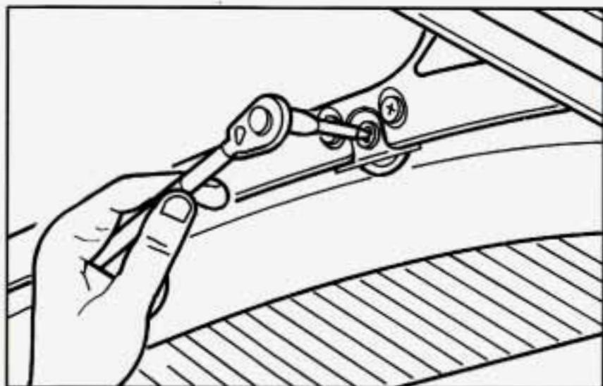
4. The two rear bolts are on the roof, one above each seat. You'll see three bolts on each side. Loosen the middle one. (The ratchet won't work for the other two.) The bolts will stay in the roof panel.
