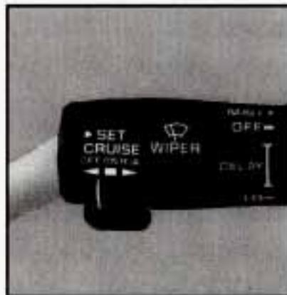
3. Push in the SET button at the end of the lever and release it.
