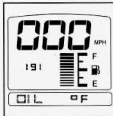
For numeric gauge measurements, press the GAUGES button on the trip monitor until OIL appears.
