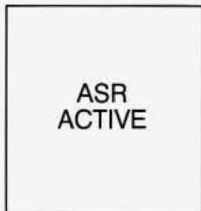
When your ASR system is limiting wheel spin, this light will come on. Slippery road conditions may exist if the ASR system active light comes on, so adjust your driving accordingly.
