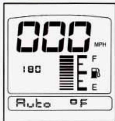
Automatic transmission fluid temperature will be displayed if you press the GAUGES button on the trip monitor until AUTO appears.
