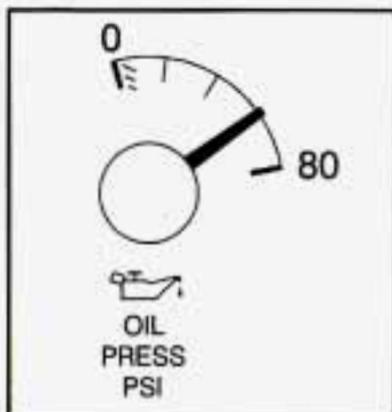
The engine oil pressure gauge shows the engine oil pressure in psi (pounds per square inch) or kPa (kilopascals) when the engine is running.
