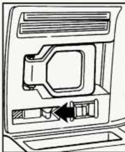
To lock the door from the inside, move the lock control on the door backward. To unlock it, move the lock control on the door forward.
