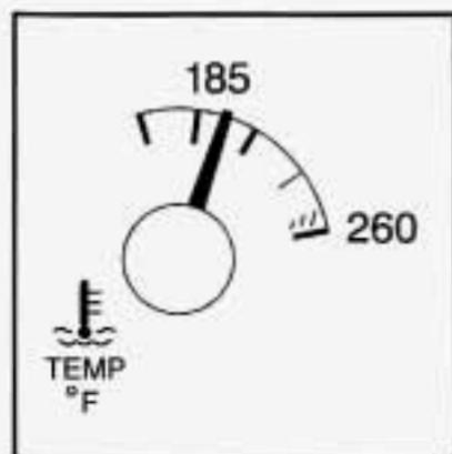
This gauge shows the engine coolant temperature. If the gauge pointer moves into the shaded area, your engine is too hot!
