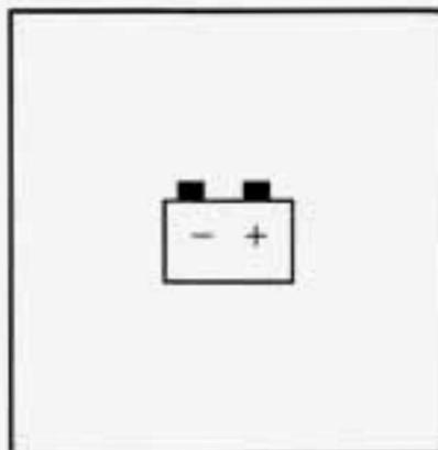
This light will come on when you turn on the ignition, but the engine is not running, as a check to show you it is working. It should go out when the engine starts.
