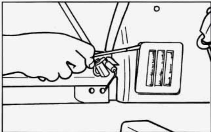
1. Pry the cover off with a screwdriver. Be sure to pry from the rear side, or you could break the tab on the cover.
