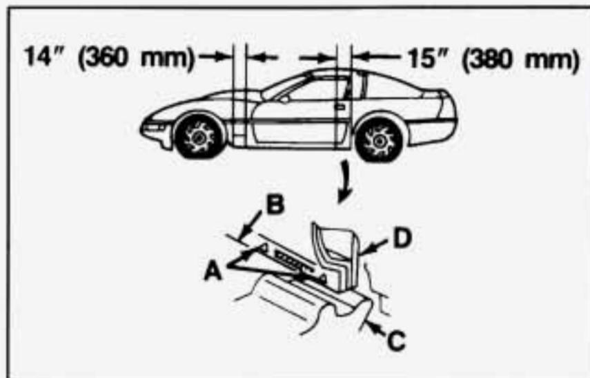
6. Position the jack under the vehicle. There are two locator triangles (A) on the panels (B) near each wheel. Raise the lift head (C) until it fits firmly under the steel rocker flange (D) between the triangles nearest the flat tire.
