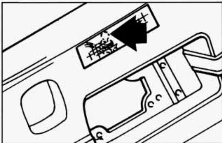
You can reach the center high-mounted stoplamp by removing the license plate and reaching through the opening.
