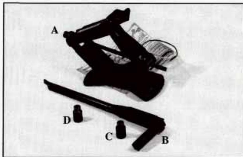
The tools you'll be using include the jack (A), wheel wrench (B), wheel nut socket (C) and wheel lock key (D).
