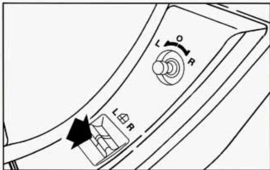
With power windows, switches on the door control each window when the ignition is on or when DAB is present. (See “Delayed Accessory Bus” in the Index.)
