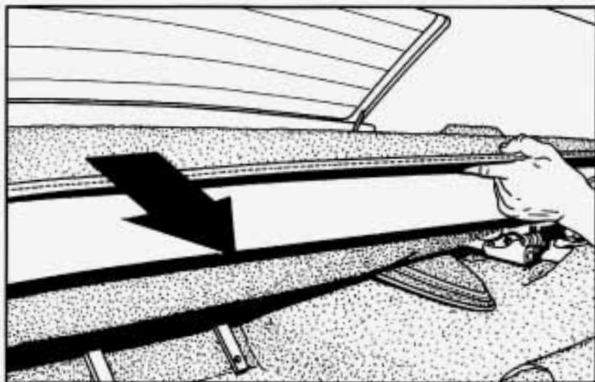
3. Move both seatbacks forward and remove the rear trim panel.
