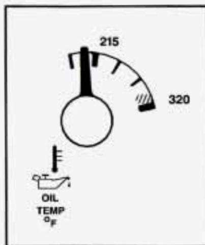
This gauge shows your engine oil temperature. Oil temperature may vary with the type of driving you do and weather conditions.
