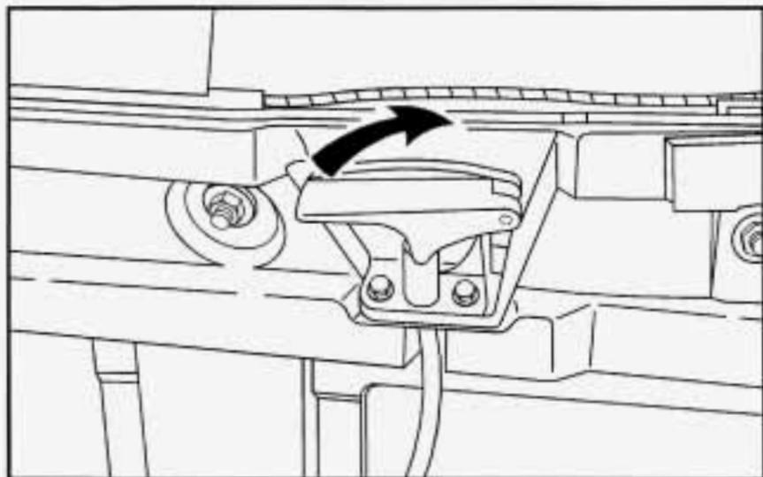
4. Tilt the driver's seatback forward. The convertible top release handle is behind the driver's seat, beneath the storage compartment lid. Pull the inside edge of the handle forward.
