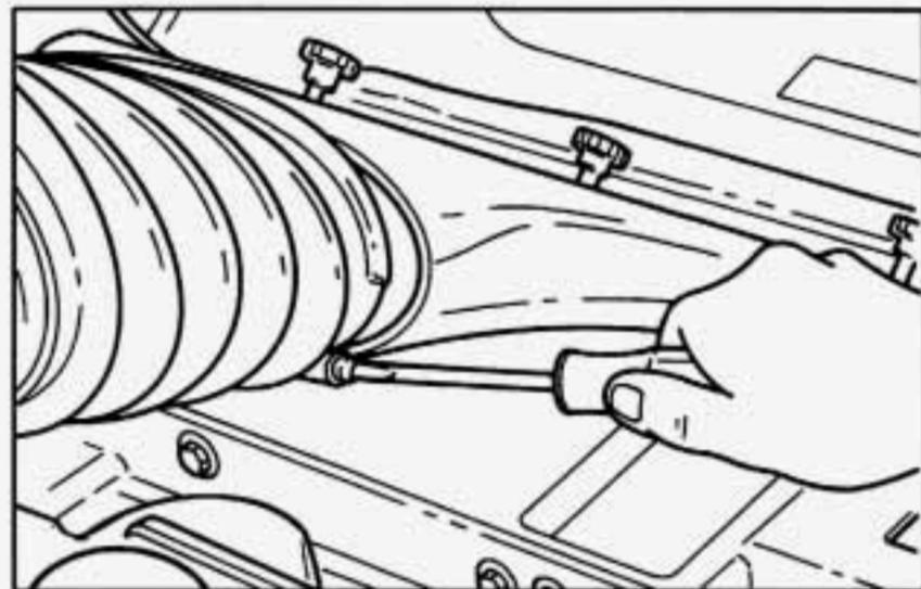
2. Disconnect the clamp from the manifold.
