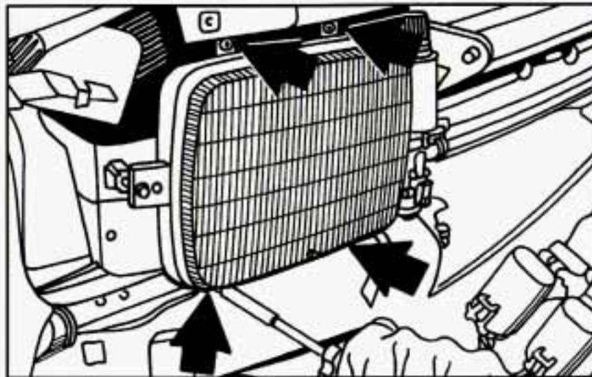
6. Remove the four screws from the retainer near each corner of the headlamp. Don't move the large-head adjusting screws or your headlamp will not be aimed properly.
