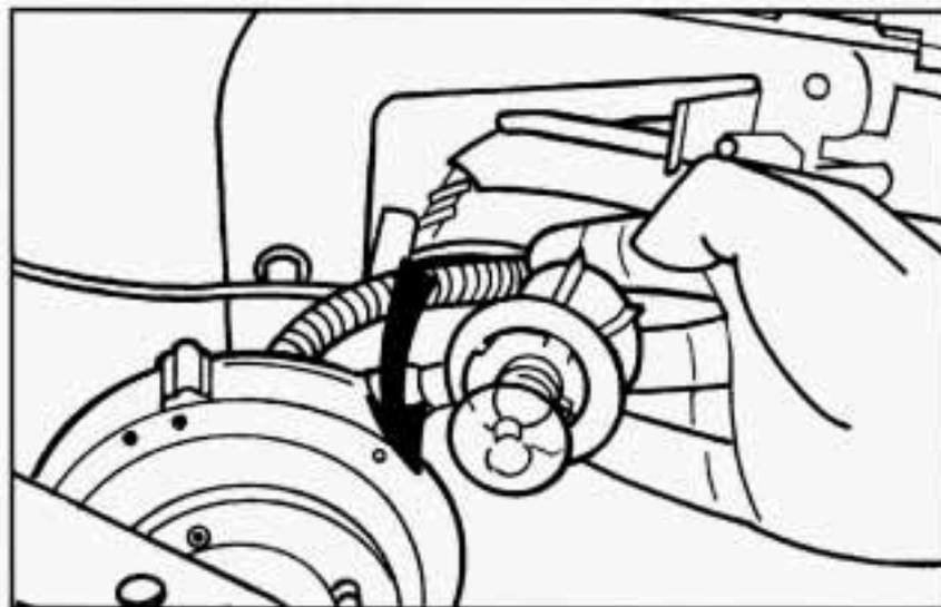
4. Push the bulb in, turn it counterclockwise, then pull it out.
