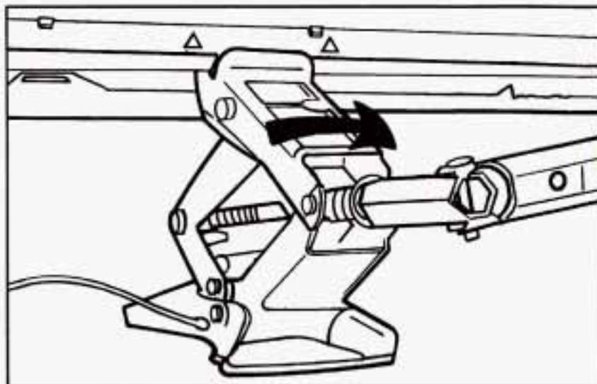
7. Raise the vehicle by turning the wheel wrench clockwise. Raise the vehicle far enough off the ground so there is enough room for the spare tire to fit. Remove all the wheel nuts and take off the flat tire.
