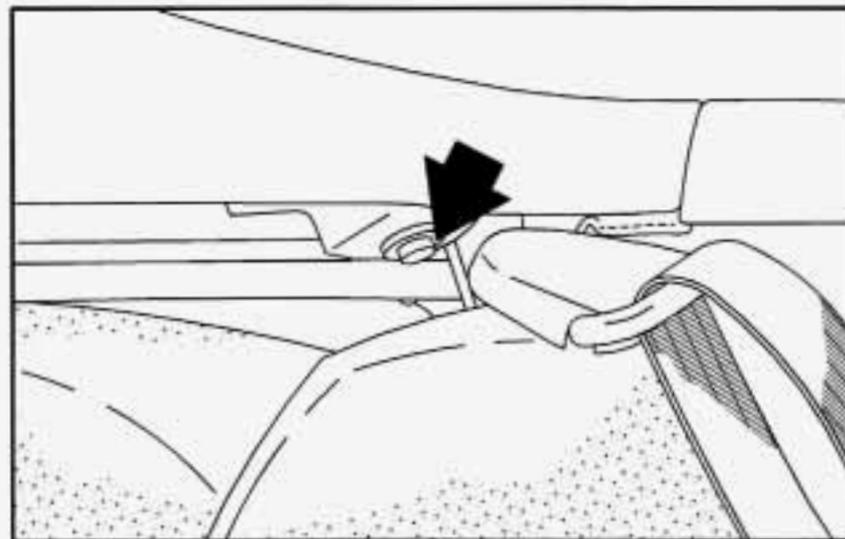
5. From the driver's side, lift and hold the rear of the top with your left hand. With your right hand, press the storage compartment lid release button behind the driver's seat on the lid (the release switch in the center console will also work). Raise the lid.
