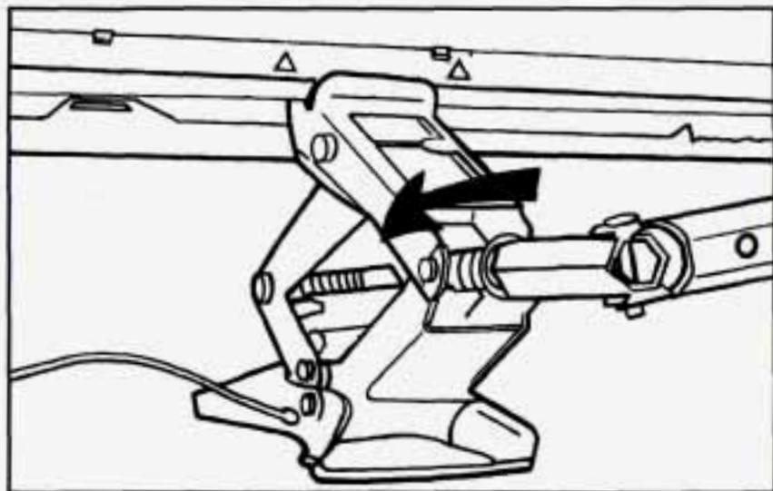
10. Lower the vehicle by turning the wheel wrench counterclockwise. Lower the jack completely.
