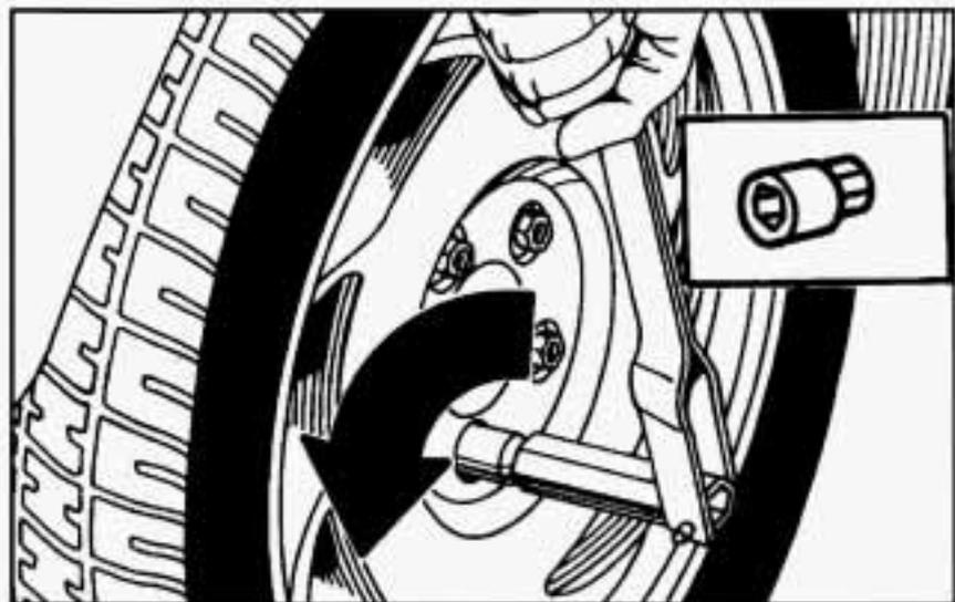
3. Attach the wheel nut socket to the wheel wrench and loosen all the wheel nuts by turning the wrench in the direction shown. Don't remove them yet.
