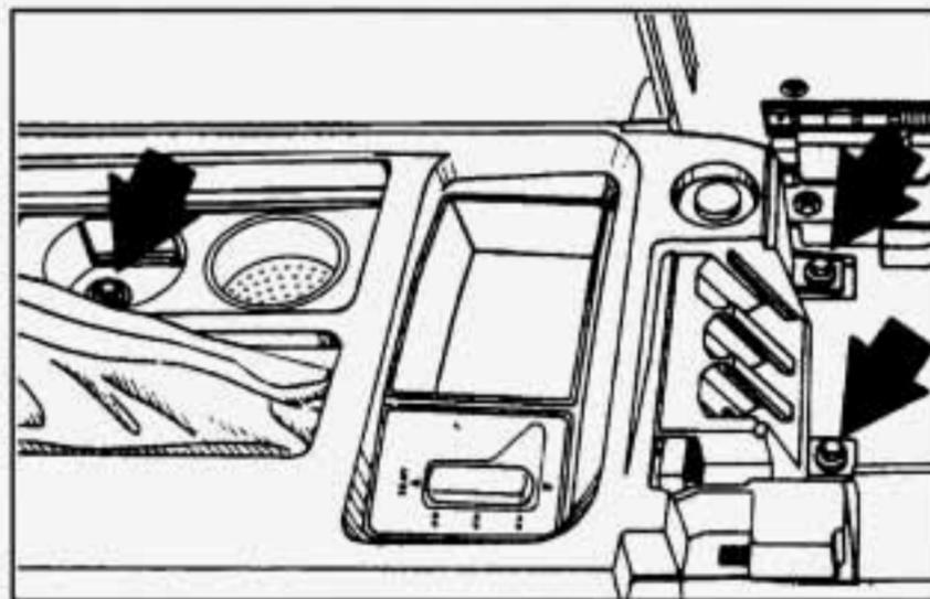
3. Open the ashtray door, remove the ashtray and the rubber insert from the forward location, and remove the screw inside the cupholder.
