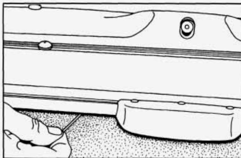
If you don't have battery power, use the manual release cable to open the hatch. The cable is near the security shade handle, between the carpet and the shade.
