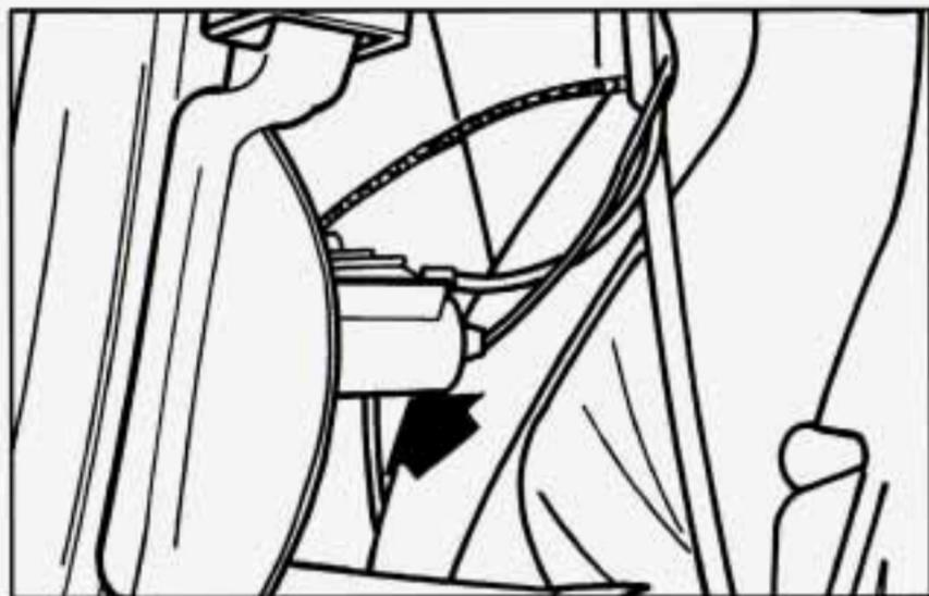
You can reach the back-up lamps by removing the license plate and reaching through the opening.
